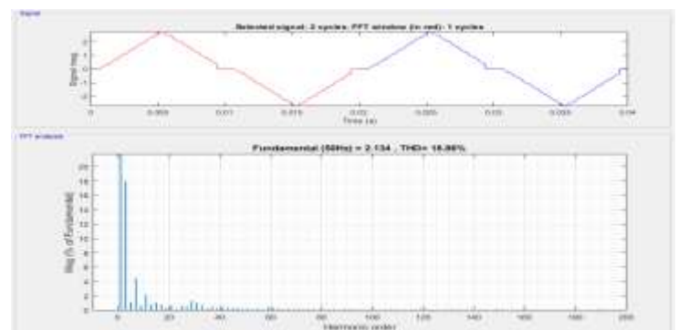
Fig. 8. THD of current waveform on RL-load using EPM
