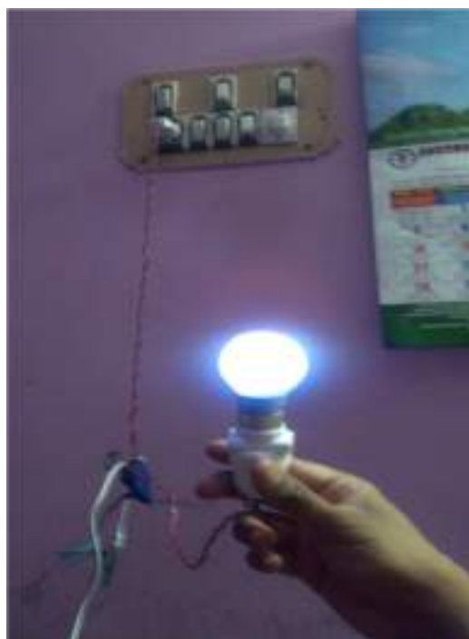
Figure 8: Switch ON button in Blynk App and Light ON
