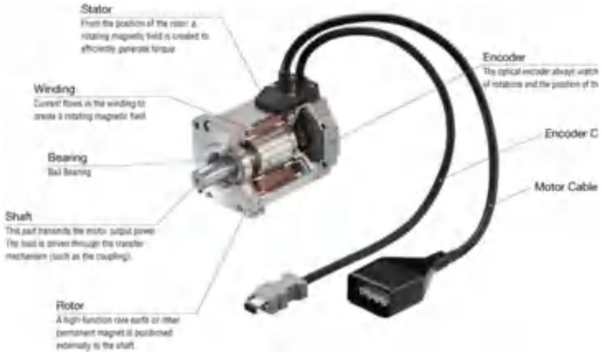
Fig. 5 Servomotor structure
